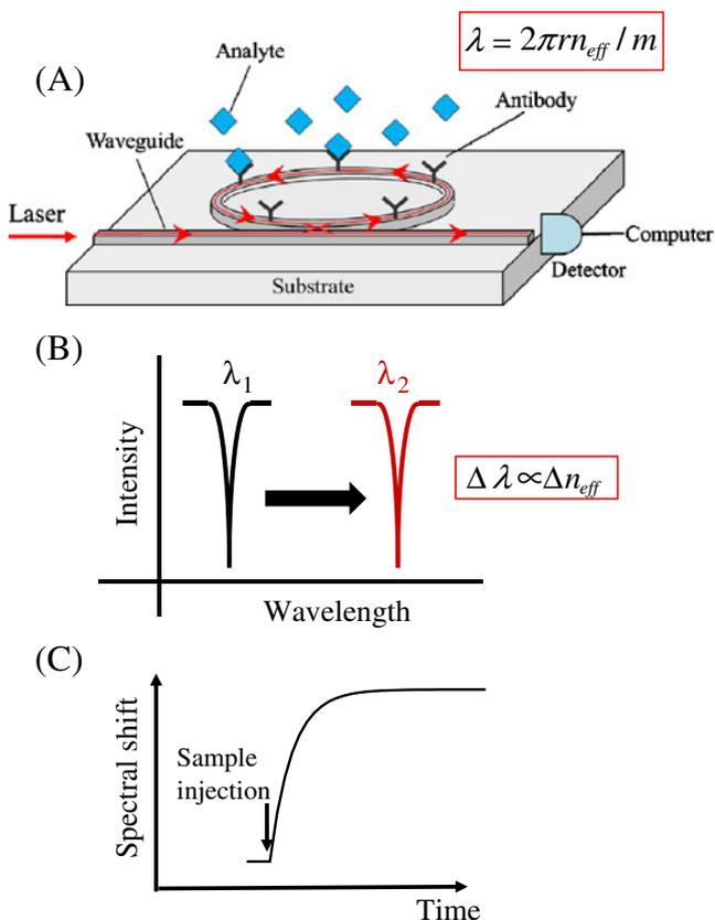
**Fig. 3** (a) Illustration of a ring resonator biosensor that detects the binding of analyte to the surface. A tunable laser is coupled to the ring resonator. When the laser is in resonance with the resonant mode in the resonator, a spectral dip is shown at the detector to indicate the spectral position. (b) The resonant mode shifts in response to the local RI change induced by the molecular binding. (c) A sensorgram can be obtained by monitoring the spectral shift in real time
