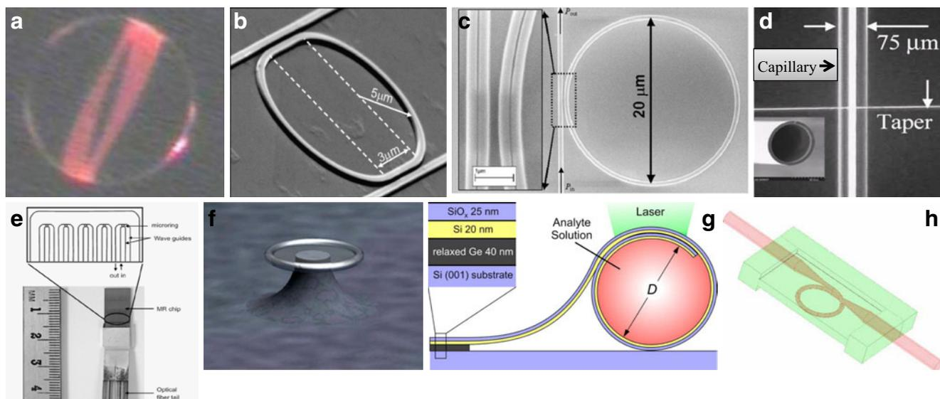
**Fig. 2** Various ring resonator sensor configurations. (a) Microsphere. (b) Silicon-on-insulator planar ring resonator. (c) Slot waveguide ring resonator. (d) Capillary-based ring resonator fabricated by the drawing method. (e) Planar ring resonator array. (f) Microtoroid. (g) Capillary-
