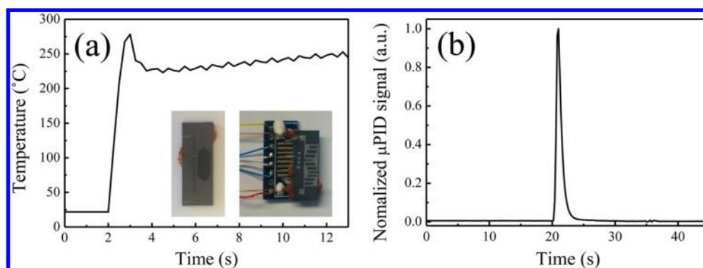
**Figure 3.** (a) Temperature response of the  $\mu$ PI. The  $\mu$ PI reached 270 °C in 0.6 s and then kept at 250 °C for 10 s. Inset shows the front and back side of the  $\mu$ PI packed with CarboPack B. At the back side, the heater and resistive temperature detector (RTD) were wire-bonded to a printed circuit board. (b) Normalized toluene peak obtained by PID 1 under the injection condition of part a. The helium flow rate was 2 mL/min, fwhm = 700 ms.
