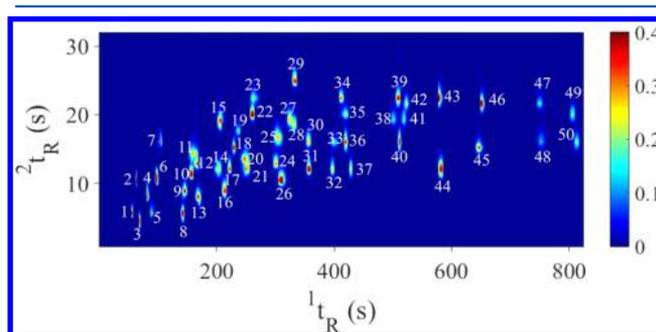
**Figure 6.** 2-D contour plot of the 50 VOCs generated with the portable  $1 \times 4$ -channel GC  $\times$  GC device. The list of those VOCs is given in Table S1.
