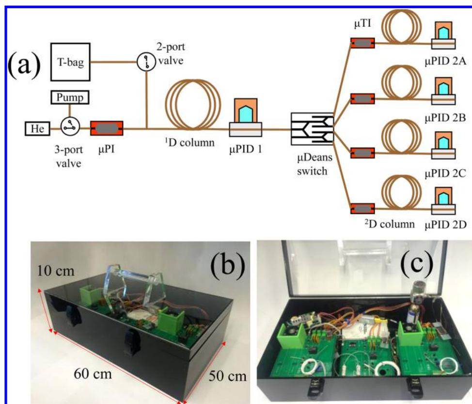
**Figure 1.** (a) Schematic of the portable 1 × 4-channel GC × GC device. (b and c) Photos of outside and inside of the device. The detailed device layout is shown in Figure S1.
