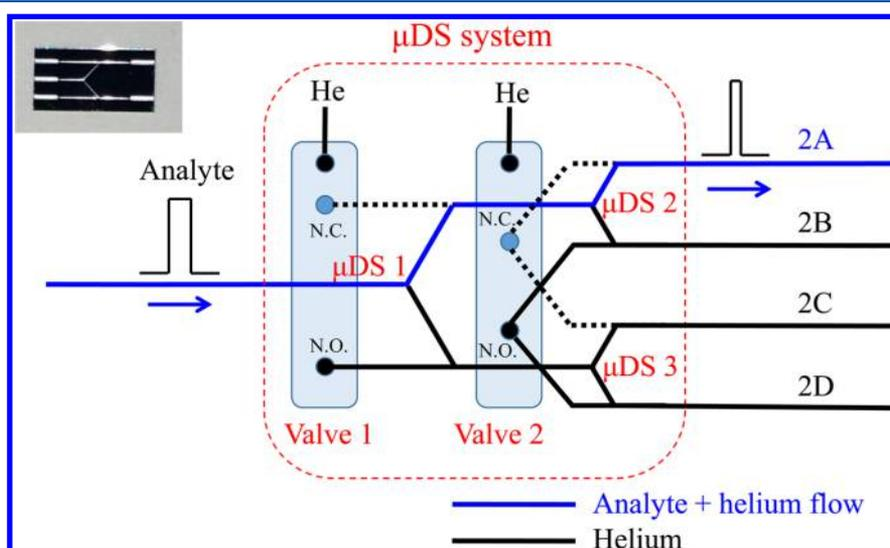
**Figure 4.** Schematic of the  $1 \times 4$  flow switching module consisting of three  $\mu$ DSs (see the  $\mu$ DS picture in the inset) and two 3-port valves. The figure shows that the analyte is routed from the  $^1$ D column to Column 2A in  $^2$ D. The detailed  $\mu$ DS dimensions and the flow switching operation can be found in Figures S3 and S4.
