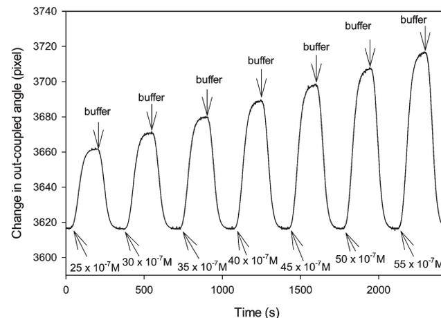
Fig. 4 The response of the TE<sub>0</sub> mode to different concentrations of paraoxon (data smoothed for clarity).
