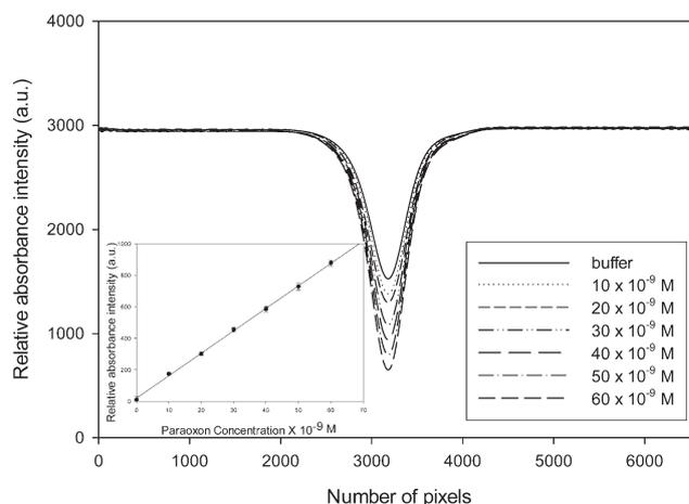
**Fig. 7** The change in the TE<sub>0</sub> solvent blue-CLW mode intensity and the calibration curve for different concentrations of paraoxon. Error bars represent  $\pm 1$  standard deviation,  $n = 4$ .
