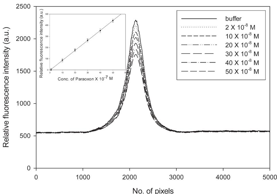
**Fig. 8** The decrease in the fluorescence of FITC-labelled OPH TE<sub>0</sub> mode of PT-CLW and the calibration curve for different concentrations of paraoxon. Error bars represent  $\pm 1$  standard deviation,  $n = 4$ .
