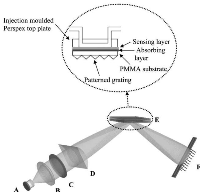
**Fig. 2** Sensor optical design using (a) 473 nm LED or 610 nm LED, (b) collimating lens, (c) filter, (d) cylindrical lens, (e) sensor chip, (f) linear CCD detector.
