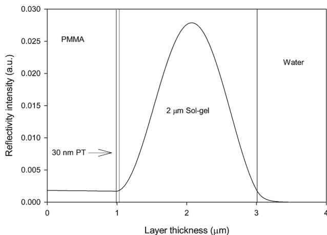
Fig. 1 Mode profile of PT-CLW at 470 nm.
