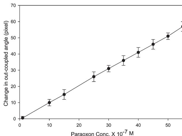
**Fig. 6** Calibration curve of the paraoxon TE<sub>0</sub> mode of the solvent blue-CLW to various concentrations of paraoxon. Error bars represent  $\pm 1$  standard deviation,  $n = 5$ .
