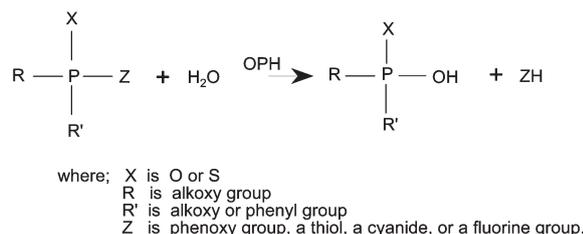
Fig. 3 Catalytic reaction of OPH.<sup>11,62</sup>
