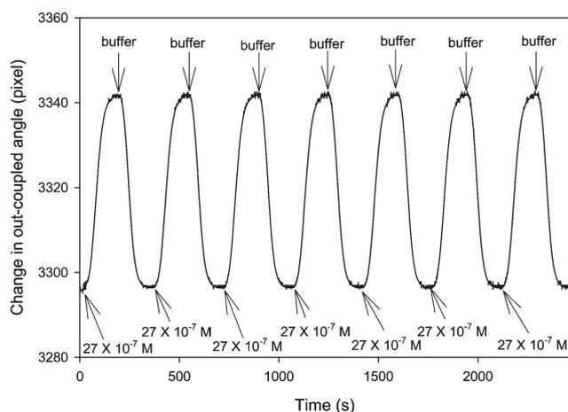
**Fig. 5** Reproducibility of the TE<sub>0</sub> mode of the solvent blue-CLW for  $27 \times 10^{-7}$  M paraoxon (data smoothed for clarity).
